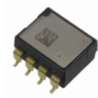
SCA610-CA1H1G-1 Murata Electronics North America INCLINOMETER 1-AXIS 90DEG 8SMD
