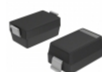
MMSZ5235B Fairchild/ON Semiconductor DIODE ZENER 6.8V 500MW SOD123
