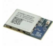
ATSAMB11-MR210CA Microchip Technology RF TXRX MOD BLUETOOTH CHIP ANT
