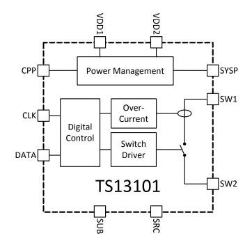
Figure 1: TS13101 Block Diagram
