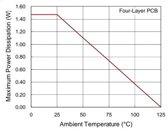
Figure 8. Derating Curve for RT8510 Package
