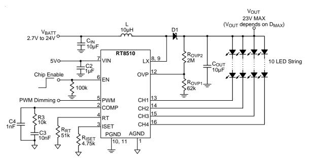
Figure 2. Low Input Voltage Application Circuit
