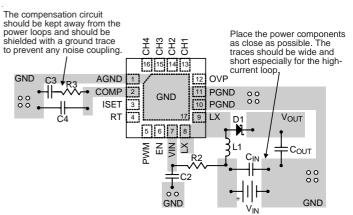
Figure 9. PCB Layout Guide
