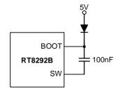
Figure 2. External Bootstrap Diode
