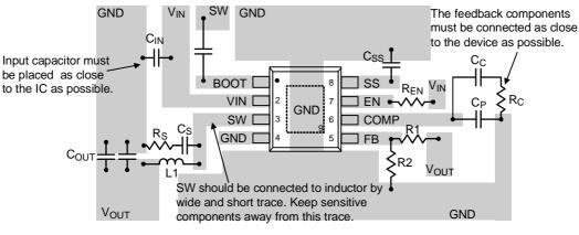
Figure 8. PCB Layout Guide
