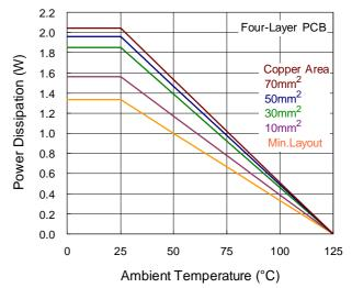
Figure 7. Derating Curves for RT8292B Package
