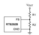
Figure 1. Output Voltage Setting
