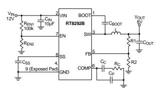
Figure 4. The Resistors can be Selected to Set IC Lockout Threshold
