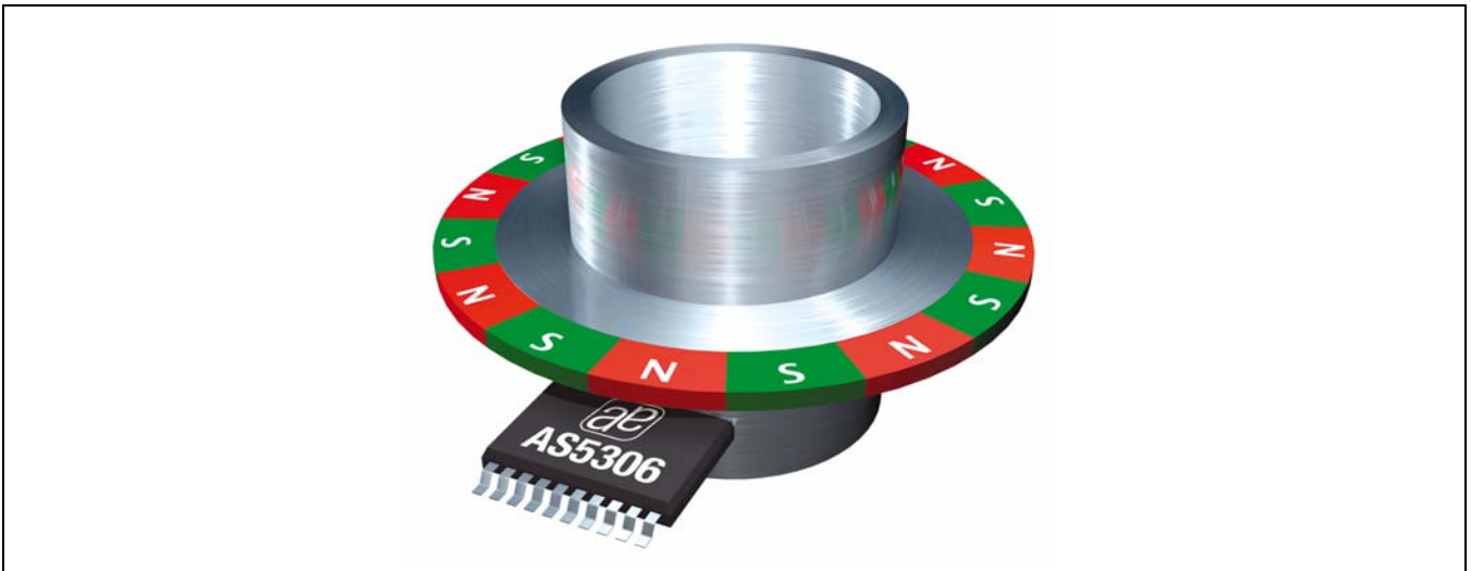
Figure 1 AS5306 with multipole ring magnet for off-axis rotary motion sensing (not to scale)
