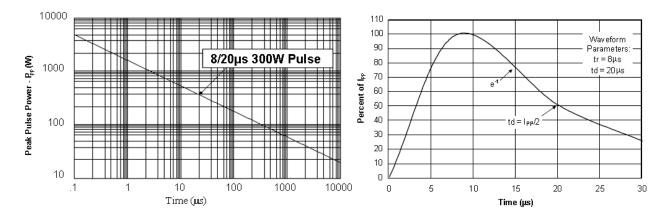
Figure 1. Peak Pulse Power Vs Pulse Time ( $\mu s$ )
