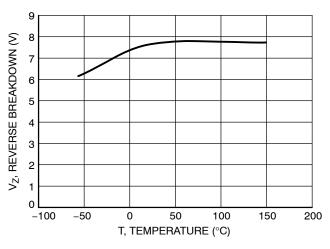
Figure 1. Reverse Breakdown versus Temperature
