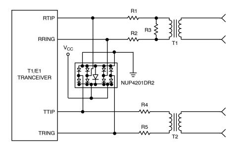
Figure 14. TI/E1 Interface Protection
