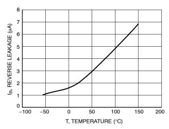
Figure 2. Reverse Leakage versus Temperature
