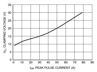
Figure 4. Clamping Voltage versus Peak Pulse Current
