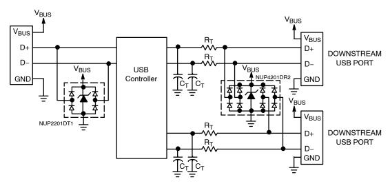
Figure 12. ESD Protection for USB Port
