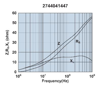
Impedance, reactance, and resistance vs. frequency.
