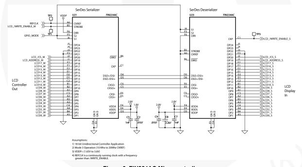
Figure 6. FIN224AC Microcontroller
