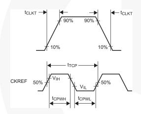
Figure 9. LVCMOS Clock Parameters
