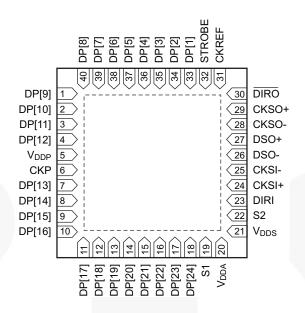
Figure 3. Terminal Assignments for MLP (Top View)
