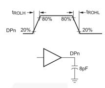
Figure 7. LVCMOS Output Load and Transition Times
