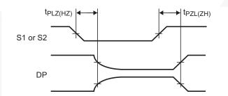
Note: If S1(2) transitioning then S2(1) must = 0 for test to be valid
