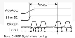
Figure 11. Serializer PLL Lock Time
