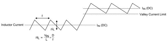
Figure 5. Inductor Currents In Current Limit Operation
