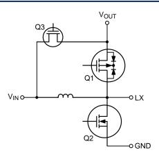
Figure 2. Boost Converter With Bypass Mode
