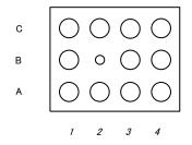
Figure 2. Pin assignment (Bottom view)
