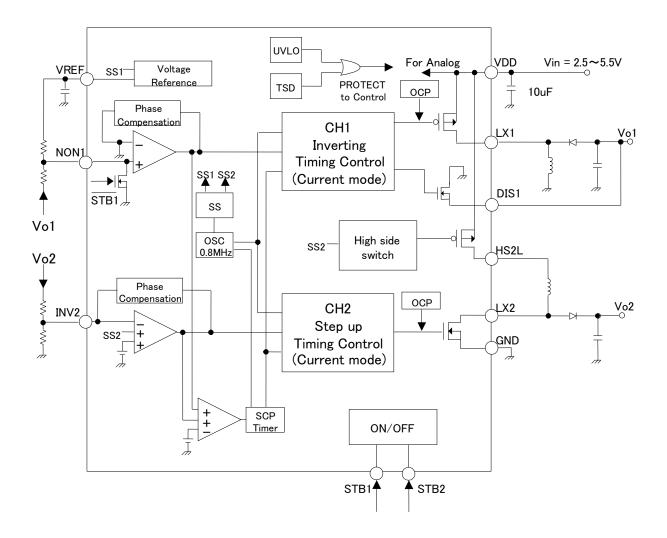
Figure 3. Block diagram
