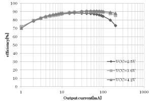
Figure 21. CH2 Power conversion efficiency vs output current
