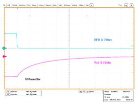
Figure 30. CH1 Discharge waveform [500usec/div]
