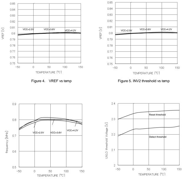
Figure 6. Oscillation frequency vs temp
