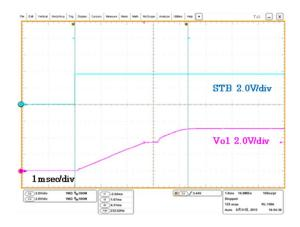
Figure 29. CH2 Soft start waveform
