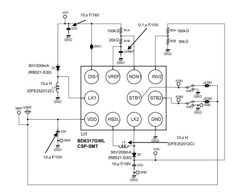
● Example of Application1 Input: 2.5 to 5.5 V, ch1 output: -5.0 V / 100m A(MAX), ch2 output: 5.0 V/100mA(MAX)
