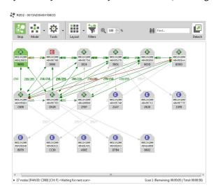
3. The scan process automatically stops according to the network preferences configured in Set network discovery preferences. You can also click **Stop scanning the network** at any time.
