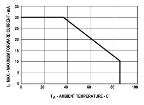
Figure 5. Maximum Fwd. Current vs Temperature
