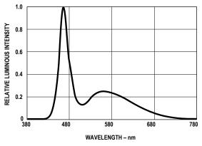
Figure 1. Relative Intensity vs Wavelength
