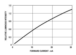
Figure 3. Relative Iv vs. Forward Current
