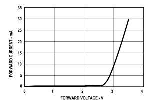
Figure 2. Forward Current vs Forward Voltage
