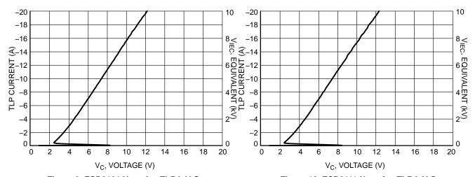
Figure 9. ESD8101 Negative TLP I-V Curve
