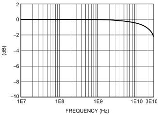
Figure 3. ESD8101 S21 Insertion Loss
