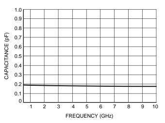
Figure 5. ESD8101 Capacitance over Frequency
