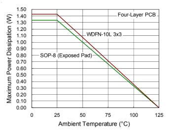
Figure 2. Derating Curves for RT8068A Packages
